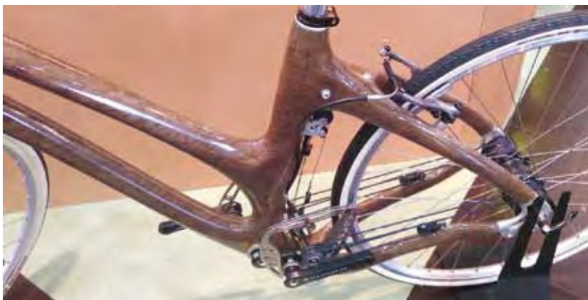
Figure 1. Bike frame made out of natural fibre composites
