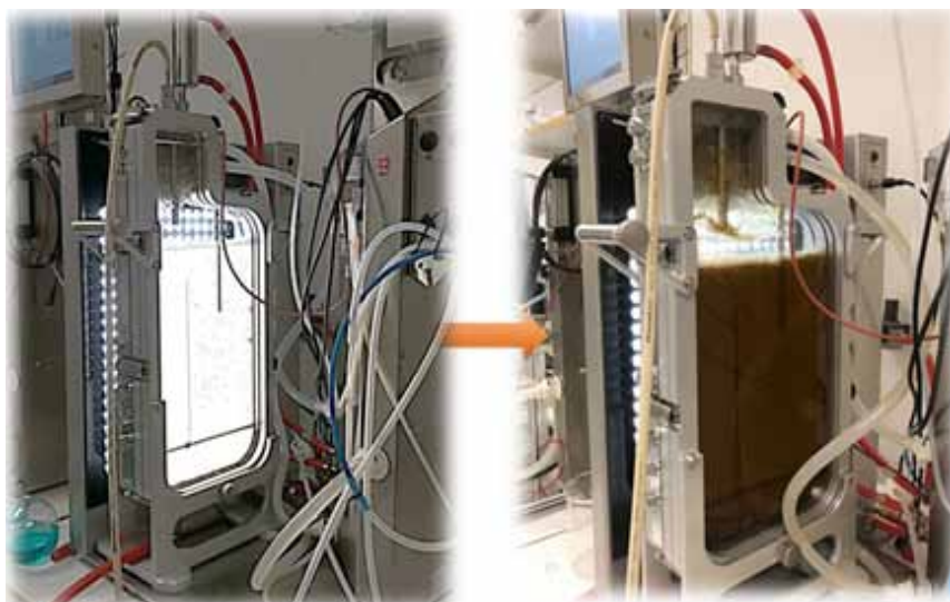
Figure 3: Cultivation of microalgae on hydrolyzed cellulose for the production of omega-3 PUFAs. The figure is reprinted from Patel et al [20] under the CC BY 4.0 license.
